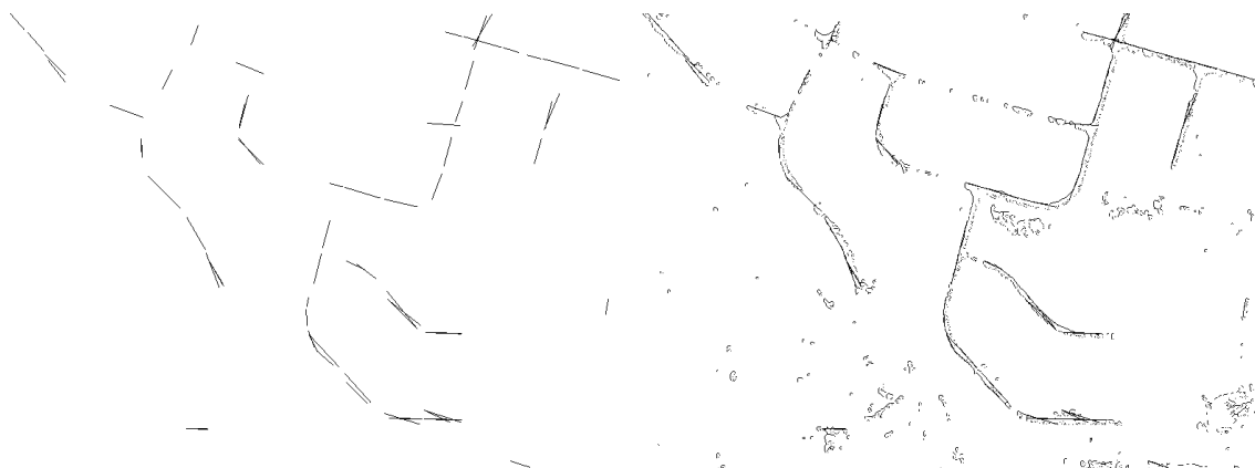
Figure 6: The Block-Based Hough Transform before line joining is done
