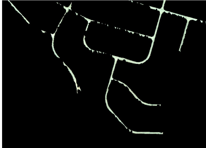
Figure 2: The modified input image - the black area has an alpha value of 0, while the roads have a value of 1
