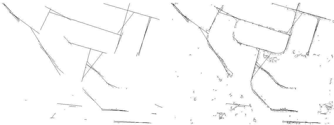
Figure 3: An example of the Hough Transform using the single pixel checker
