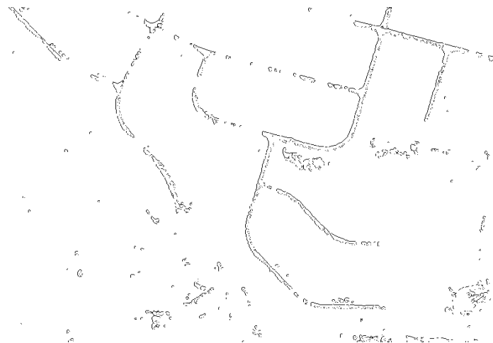
Figure 10: An example of RGB-based directed edge detection
