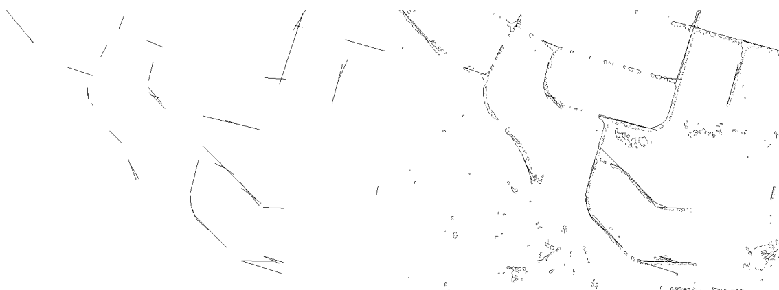
Figure 7: The Block-Based Hough Transform after line joining
